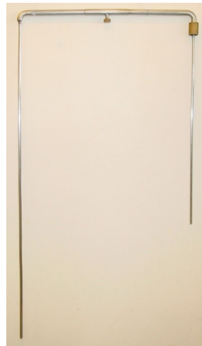
Helium vacuum-insulated transfer line
